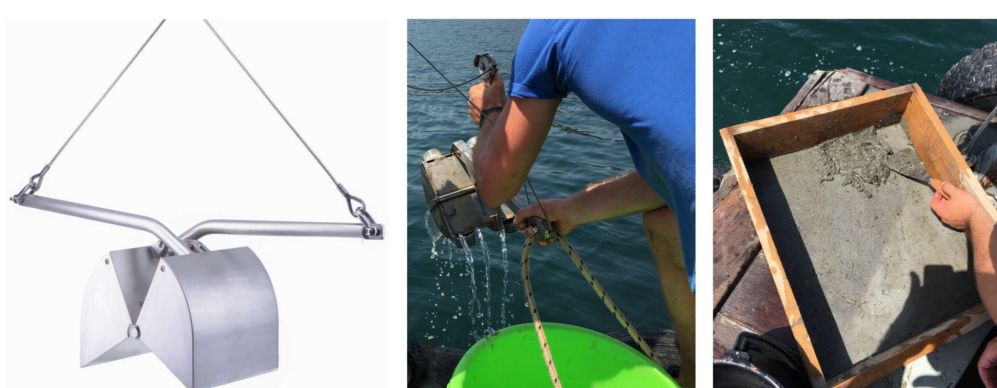
Fig. 2. The sediment samples were collected with a Van Veen grab and were sieved on-board with a 0.5 mm mesh-size sieve.
